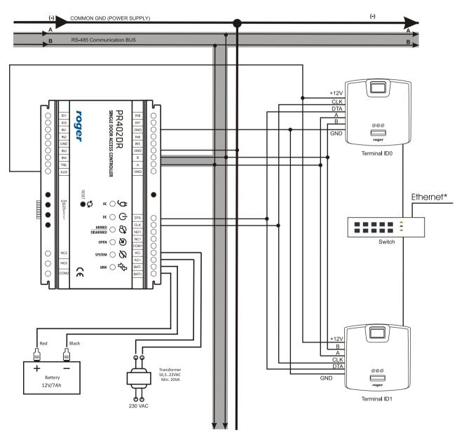
\* NOTE! If the system is operated by means of Ethernet port then RS485 bus is not used for communication with RFT1000 readers.
