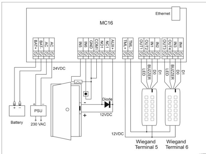
Fig. 2 Typical door control with Wiegand readers
