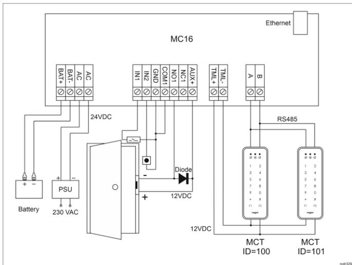
Fig. 2 Typical door control with MCT readers
