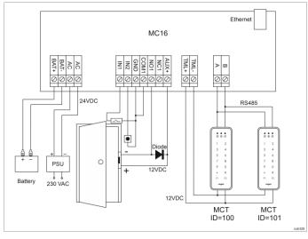
Fig. 2 Typical door control with MCT readers
