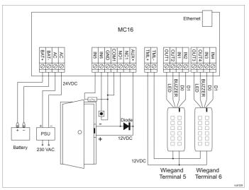
Fig. 2 Typical door control with Wiegand readers
