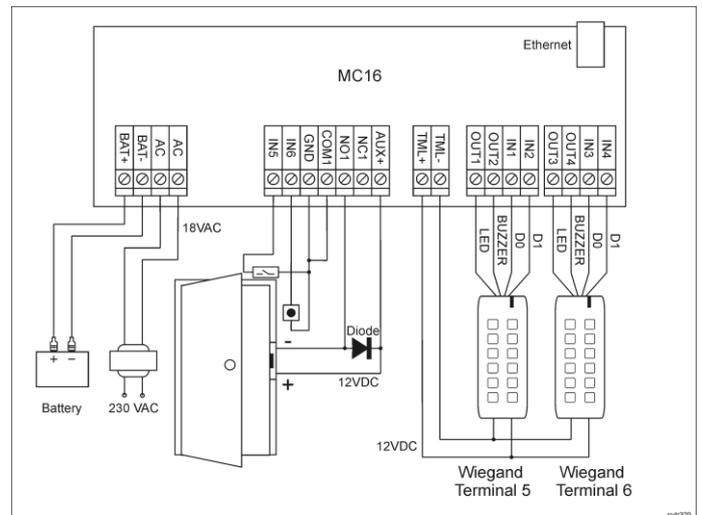
Fig. 4 Typical door control with Wiegand readers
