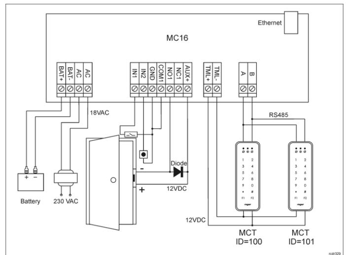
Fig. 3 Typical door control with MCT readers
