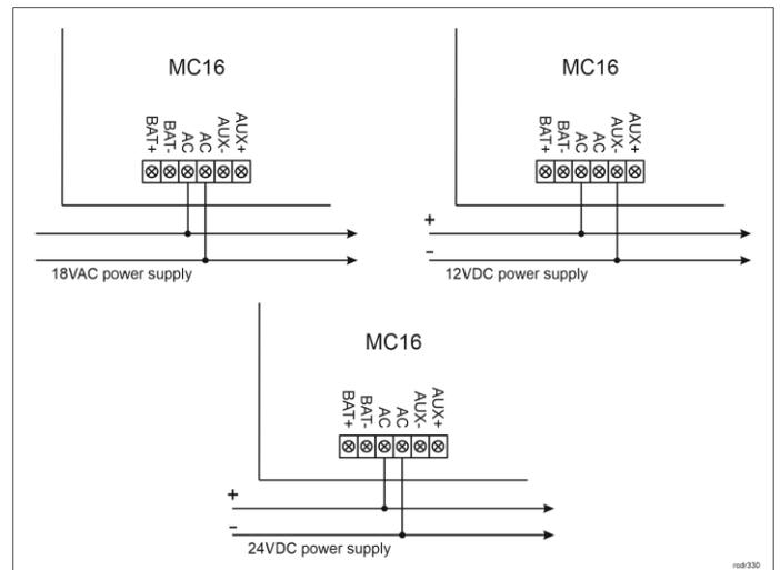
Fig. 1 MC16 power supply
