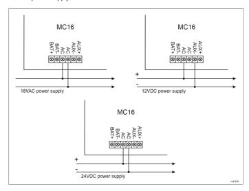
Fig. 1 MC16 power supply
