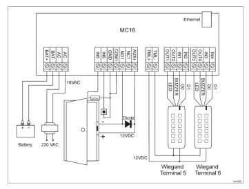
Fig. 4 Typical door control with Wiegand readers
