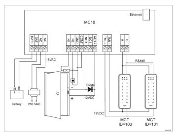
Fig. 3 Typical door control with MCT readers
