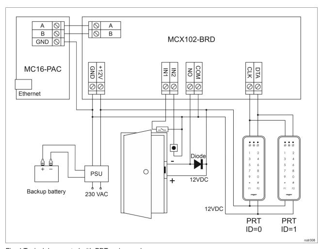
Fig. 4 Typical door control with PRT series readers
