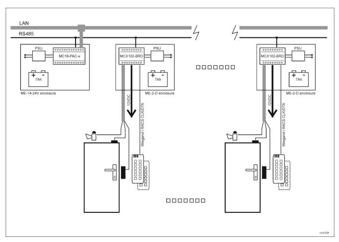
Fig. 3 Scenario of operation with MCX102-BRD expanders
