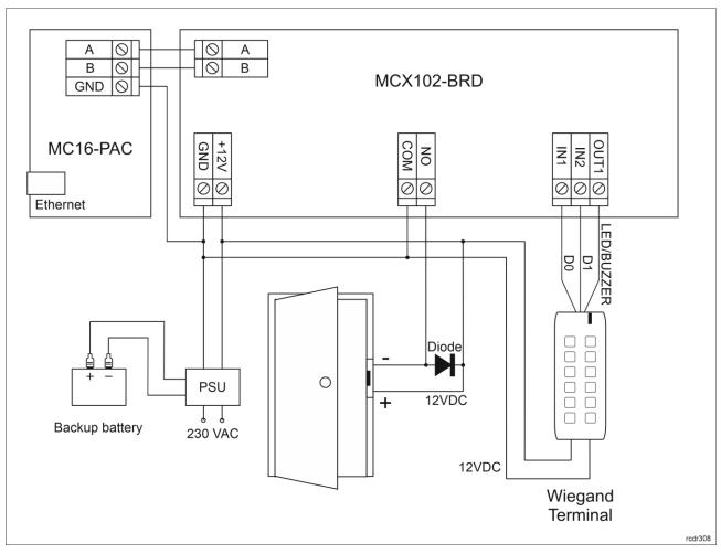
Fig. 5 Typical door control with Wiegand interface reader
