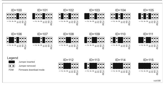
Fig. 7 Manual addressing of expander
