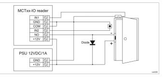
Fig. 5 Connection of door lock, door contact and exit button to MCTxx-IO reader
