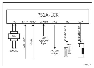
Fig. 1 Functional diagram of PS1A-LCK module
