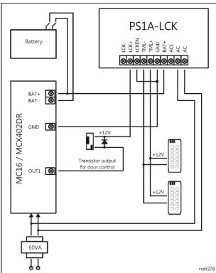
Fig. 4 Typical scenarios of door lock control with PS1A-LCK
