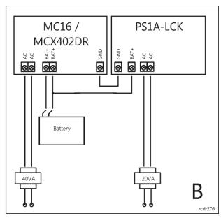
Fig 3. PS1A-LCK power supply from single transformer (A) or two transformers (B)
