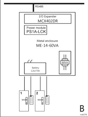
Fig. 2 PS1A-LCK installation with MC16 access controller (A) and MCX402DR expander (B)
