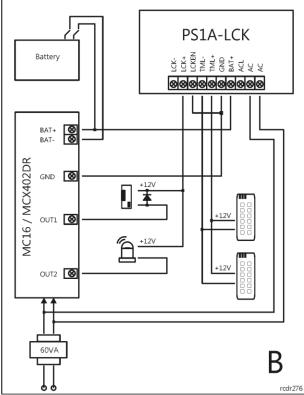
Fig. 5 Door lock and alarm signalling device (siren) control with relays (A) or transistor outputs (B)
