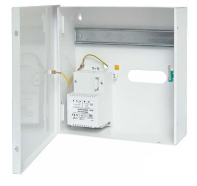
The ME-14-40VA enclosure is dedicated to RACS 5 modules and devices which require installation on DIN rail and 7 Ah battery. The enclosure is equipped with single DIN rail, mains transformer and tamper contact. Access to the internal space of the enclosure is protected by a door fixed by screws. The ME-14-40VA is made from a metal sheet painted with white powder coating.
