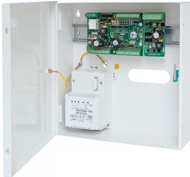
Door expander kit for two doors. The kit consists of metal enclosure with transformer, auxiliary power supply module and IO expander. The controlled doors can be managed on read-in side only by Wiegand or RACS CLK/DTA (PRT series readers) readers. Door lock and readers are supplied from the controller's on-board supply outputs
