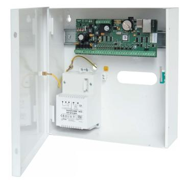
Access control kit. The kit consists of metal enclosure with transformer and MC16-RAW electronic module. With adequate license file MC16-RAW can be converted to any type of MC16 series access controller (MC16-PAC, MC16-LRC, MC16-BAC, MC16-EVK, MC16-EVC).
