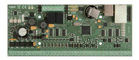
The MCX16-UZ I/O expander enables use of Clex (Uhlmann & Zacher) wireless locks as access terminals in RACS 5 system. MCX16-UZ operates as hardware interface for communication of Clex locks with MC16
