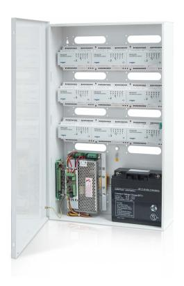
Metal enclosure with four DIN mounting rails as well as power supply unit and voltage distributor. The housing is equipped with a tamper contact and provides space for installation of 17 Ah battery. The enclosure can accommodate 9 PR402DR-12VDC controllers, 18 PR102DR or 18 HRC102DR controllers. ML-1 key lock is available as an option.
