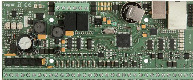
The MCX16-AP is an expander that allows connection of the Aperio by ASSA ABLOY electronic door locks to the MC16 access controller. The access rules to doors equipped with Aperio locks are determined by the configuration of the access controller which furthermore
