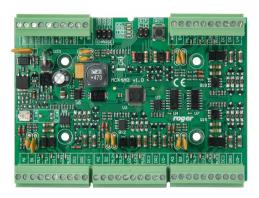
The MCX4D is an 4 door IO expander dedicated for the RACS 5 system. Apart from the IO lines, it distributes power supply and RS485 communication bus to the controlled doors. For each door it provides 2 signal inputs, 2 control outputs, 2 supply outputs and communication interface to readers. The door circuits are electrically separated what assures that in case of malfunction or sabotage, the problem which occurred on a single door is not propagated to other doors. The MCX4D is supplied
