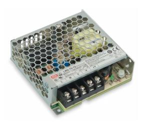
PS4D is LRS-75-12 (Mean Well) power supply unit with rated output voltage increased from 12 V to 13.8 V by means of original output potentiometer. PS4D is dedicated to installation in RACS 5 system, particularly to supply MCX2D and MCX4D expanders and PSD4D power distributors but it can also be used for other applications if its nominal conditions of use are satisfied. The PSU is
