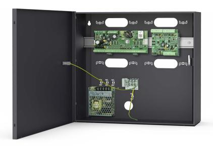
Two-door access control kit for the RACS 5 v2 EX system. The kit comprises a metal enclosure with a power supply, a door expander and a network access controller. MC16-PAC-EX-2-KIT enables the implementation of read-in/ read-out access control for two doors using RS485 (MCT series readers), RACS CLK/DTA (PRT series readers) or Wiegand readers.
