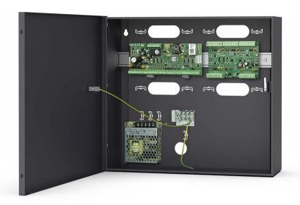
Four-door access control kit for the RACS 5 v2 ST system. The kit comprises a metal enclosure with a power supply, a door expander and a network access controller. MC16-PAC-ST-4-KIT enables the implementation of read-in/read-out access control for four doors using MCT series
