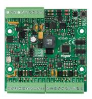
The MCX2D is an 2 door IO expander dedicated for the RACS 5 system. Apart from the IO lines, it distributes power supply and RS485 communication bus to the controlled doors. For each door it provides 2 signal inputs, 2 control outputs, 2 supply outputs and communication interface to readers. The door circuits are electrically separated what assures that in case of malfunction or sabotage, the problem which occurred on single door is not propagated to other doors. The MCX2D is supplied
