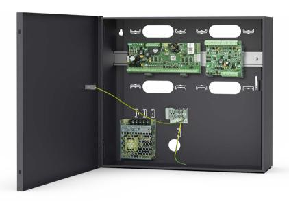
Two-door access control kit for the RACS 5 v2 ST system. The kit comprises a metal enclosure with a power supply, a door expander and a network access controller. MC16-PAC-ST-2-KIT enables the implementation of read-in/read-out access control for two doors using RS485 (MCT series readers), RACS CLK/DTA (PRT series readers) or Wiegand readers.
