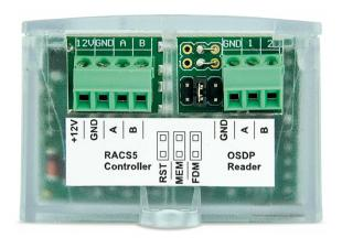
The interface enables the connection of the OSR88M-IO reader with OSDP protocol to the MC16 series access controller (RACS 5 system). The interface works as a communication converter between OSDP v2 to EPSO 3 (Roger) data transmission standards.
