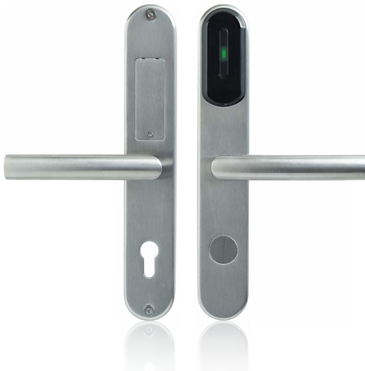
The RWL-2-SL lock enables locally managed (offline), one-way standalone access control. The lock consists of two escutcheons with handles, and it is operated on an already installed mortise lock. The card reader is installed in the external escutcheon, while the battery pack is installed in the internal one. The handle on the internal side can be permanently coupled with the latch bolt, so the door can always be opened from the
