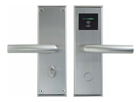
The RWL-1-SL lock enables standalone, locally configured door access. The lock consists of two escutcheons with handles and a mortise lock. The card reader is installed in the external escutcheon, while the battery pack is installed in the internal one. The handle on the internal side is permanently coupled with a deadbolt, so the door can always be opened from the inside regardless of battery state. The handle on the external side is
