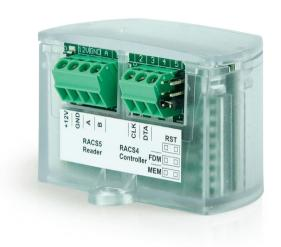
The interface enables the connection of the MCT series reader (RACS 5 system) to the PR series access controller (RACS 4 system) or the HRC series hotel controller. The interface works as a communication converter from the RS485 EPSO 3 protocol to the RACS CLK/DTA data transmission standard.
