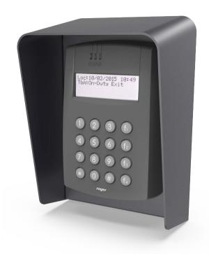
The MCT68ME-IO is a proximity reader with a keypad and built-in I/Os. The reader is designed to identify users in the RACS 5 access control system and operates with the MC16 master access controller. Communication with the controller is carried out via a modified RS485 standard, which allows star and tree-type wiring structures. The cable connection between the reader and the access controller can be up to 1200 m long and can be made
