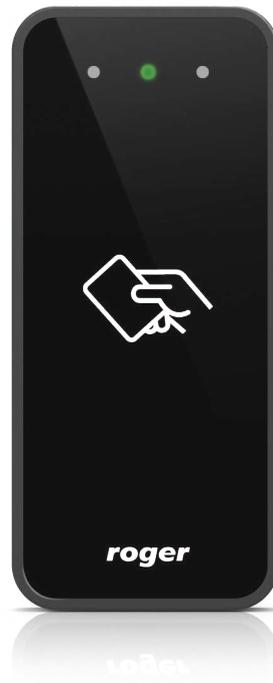
The MCT80M is an access terminal dedicated to RACS 5 access control and building automation system. Terminal enables identification of users by means of 13.56 MHz MIFARE Ultralight® and MIFARE® Classic cards. MCT80M is equipped with RS485 interface which is used for communication with access controller. Be-
