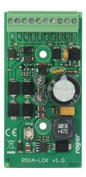
The PS1A-LCK module is supplied from 18 VAC voltage which converts into DC voltage and delivers to 2 supply outputs. The first output, 13.8 V/1.0 A rated, is dedicated to supply door lock and other access door equipment (e.g. door bell). The second output, 13.8 V/0.2 A rated, is dedicated to supply access readers. The 1.0 A output can be controlled by ON/OFF signal applied to module's input. Both outputs have overload protection.
