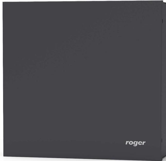
Access control kit for three doors. The kit consists of metal enclosure with power supply, networked access controller and IO expander. The controlled doors can be managed on both, read-in and read-out side, by RS485 (MCT series readers). In case the RACS CLK/DTA (PRT series readers) or Wiegand readers are used, only one door can be controlled on two sides while the remaining
