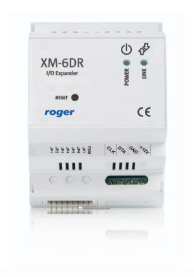
Expander with six relays, each with NO/10 A/230 VAC/30 VDC contact, RACS CLK&DTA communication interface, DIN rail plastic enclosure.
