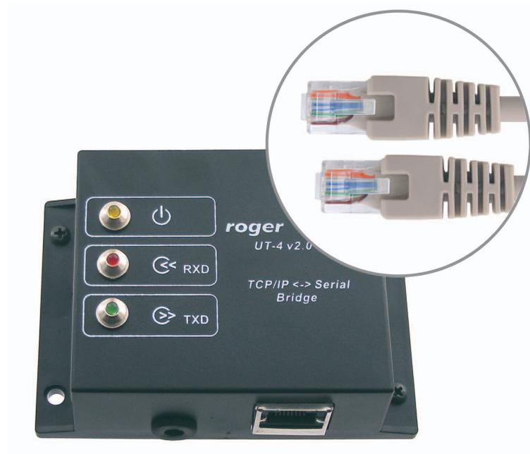
The UT-4 interface enables communication with various devices equipped with RS232 serial port through a computer network. The device is equipped with serial port which can be configured as RS232, RS422 or RS485 and with 10/100 Mb/s Ethernet port for communication within computer network.
