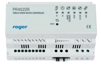
PR402DR access controllers may operate as standalone access control units or in an integrated access control system with the CPR32-SE network controller. In standalone mode, the PR402DR autonomously supervises two-way door passage and does not need to communicate with a PC or any other equipment; events are registered in their internal buffer, and time-related
