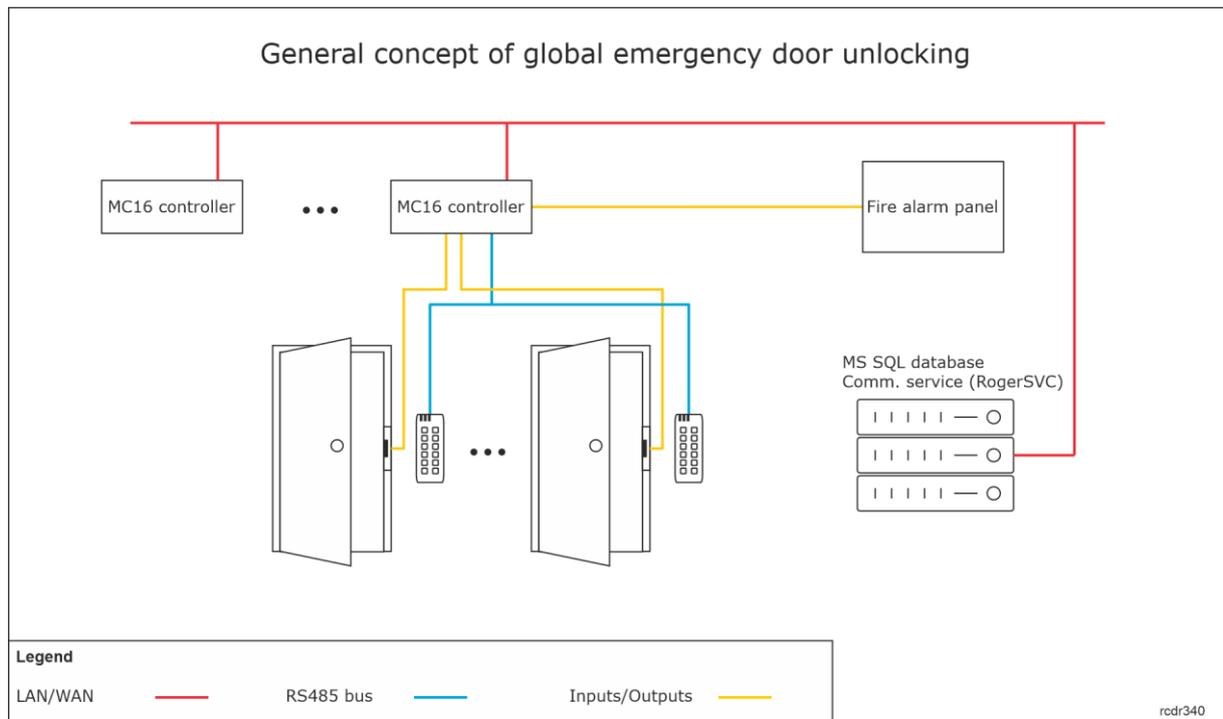
In order to configure global emergency door unlocking for RACS 5 system:
