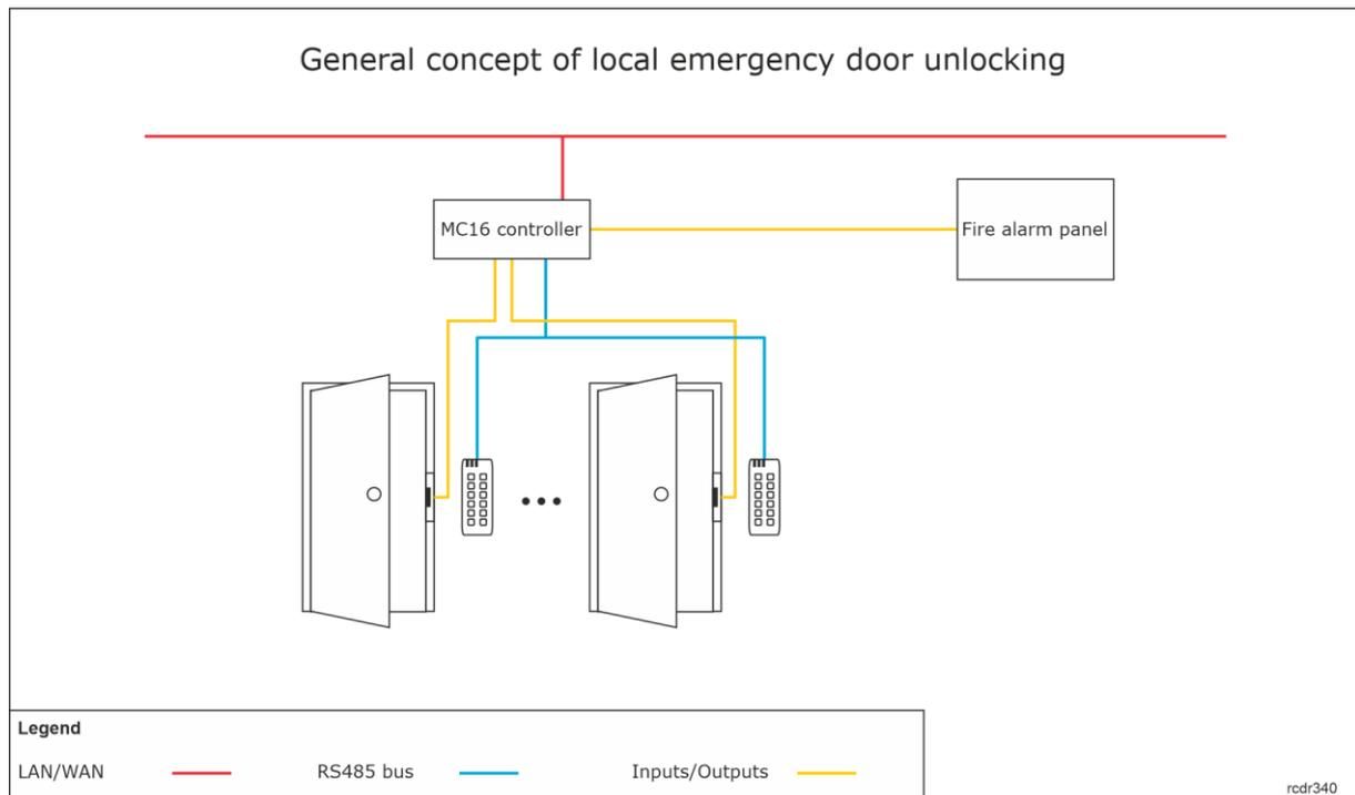
In order to configure local emergency door unlocking for MC16 controller:
