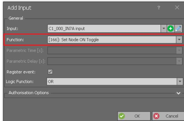
Note: Alternatively, the node can be activated and deactivated with two individual inputs respectively assigned with such functions as [161]: *Set Node ON instantly* and [163]: *Set Node OFF Instantly*. Such inputs must also be properly connected to fire alarm panel.
