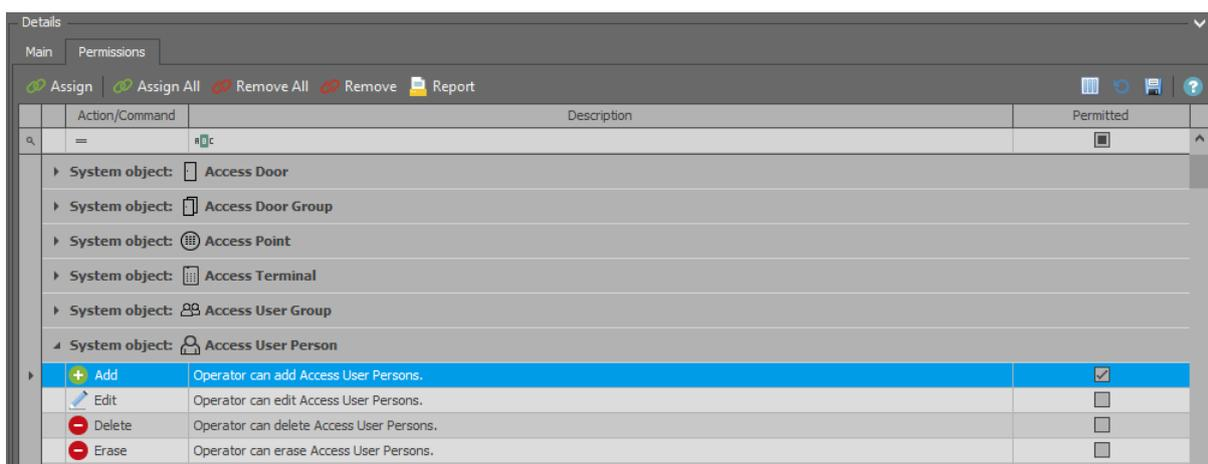
Note: Some permissions are managed in cascade. For example, access to Mainboard in VISO navigation tree requires additional access to Network and Access Controller.
