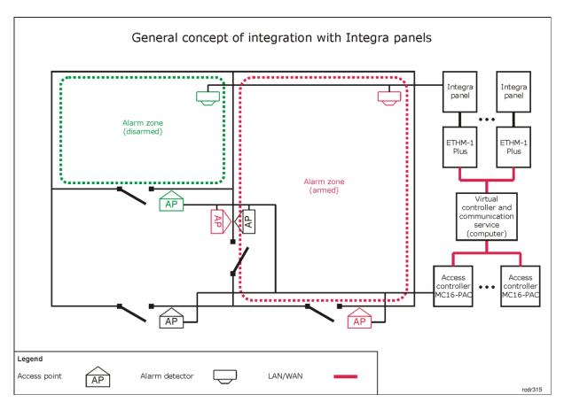
The concept of integration is based on logical connection of RACS 5 system Alarm Zones which include Access Points (readers) with Integra system Alarm Zones which include detectors. In practical application it means that the Armed mode of reader(s) and associated detector(s) is the same. Therefore the integration:
