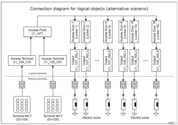
The difference between two above logic diagrams is such that depending on user Authorisations, in the first scenario each terminal can be used to control its 8 lockers while in the second scenario each terminal can be used to control any of 16 lockers. In the second scenario more than one
