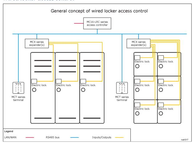
In case of wired locker access control MCT terminals are used for user identification while outputs of MCX expanders are used to control universal electric locks. The access to lockers can be provided with a single reader or lockers can be divided into groups, each with a dedicated reader.
