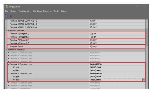
While in case of MCX402-BRD expander, configure its address on RS485 bus of MC16 controller and enable Wiegand terminals as below.
