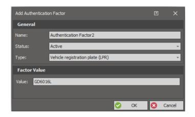
Note: It might happen that camera does not read the whole registration plate for particular vehicle. In such situation it is recommended to verify what camera reads by logging into it via web browser and using available testing tools.
