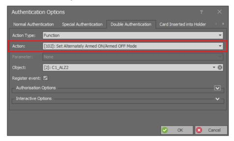
It is also possible to disarm automatically when access is granted. In such case the option *Quick Disarming* must be enabled within the properties of Alarm Zone and access authorisations as well as arming control authorisations must be assigned to user. However quick disarming can be used only in case further mentioned Method I.
