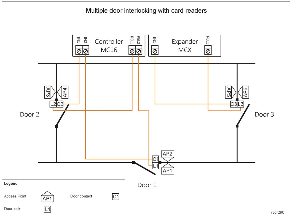
In order to configure multiple door interlocking as in example above:
