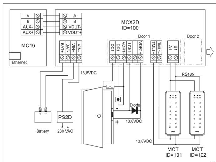
Fig. 2 Typical control of doors with MCT readers
