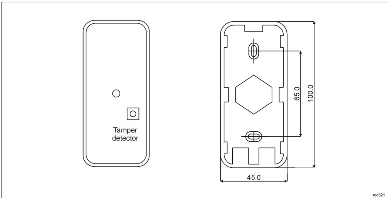
Fig. 6 Internal side of the front panel and back panel
