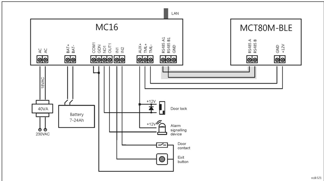
Fig. 7 Typical connection diagram for the terminal and MC16 access controller
