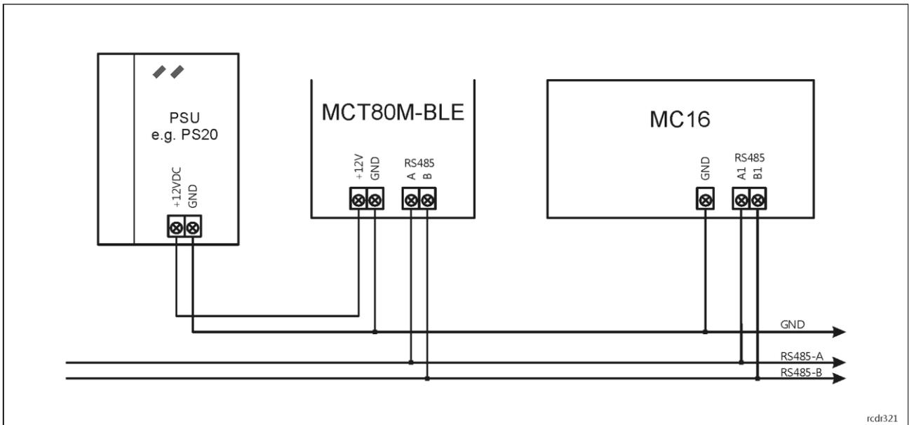
Fig. 1 MCT80M-BLE supply from dedicated power supply unit
