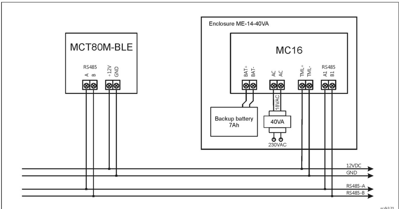
Fig. 2 MCT80M-BLE supply from MC16 access controller
