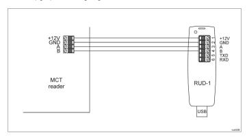
Fig. 1 Connection of MCT reader to RUD-1 interface
