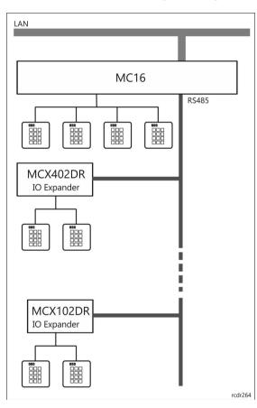
Connection of the PRT series readers to the MC16 controller
