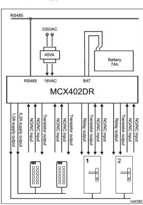
Read-in/out door control based on the MCX402 expander and Wiegand readers
