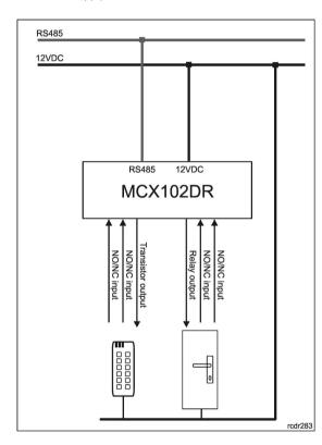
Read-in door control based on the MCX102 expander and Wiegand reader
