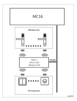
Connection of the RACS 5 AIR wireless devices to the MC16 controller
