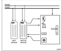
1-door control based on the MCT-IO access terminal
