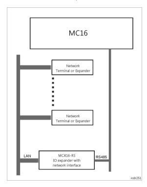
Connection of the network devices to the MC16 controller
