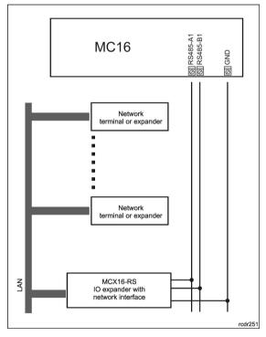
Connection of network devices to MC16 controller
