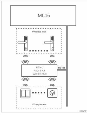
Connection of RACS 5 AIR wireless devices to MC16 controller
