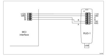
Fig. 2 Connection of the MCI-2 to RUD-1 interface for firmware update
