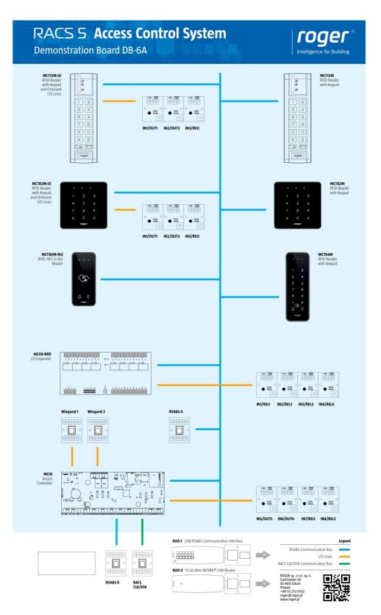
Fig.1 DB-6A functional diagram
