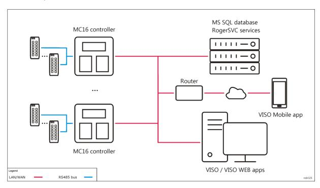
Note: In principle, the MC16 controller can be used in both WAN and LAN, while the manufacturer's warranty is covered only by working in an isolated LAN reserved exclusively for the access control system in which the controller is to be used.
