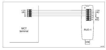
Fig. 1 Connection of MCT terminal to RUD-1 interface
