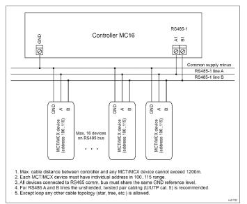
Fig. 4 Connection of terminals and expanders to MC16 access controller
