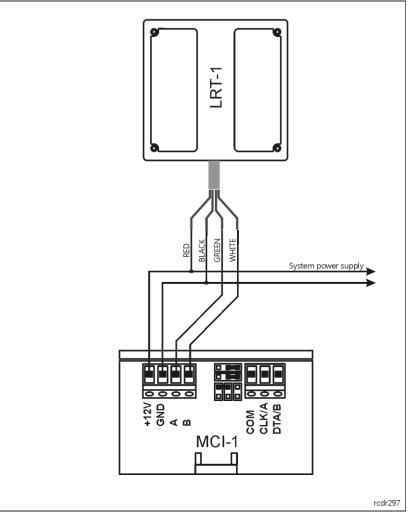
Fig. 2 LRT-1 power supply from system (e.g. from controller)
