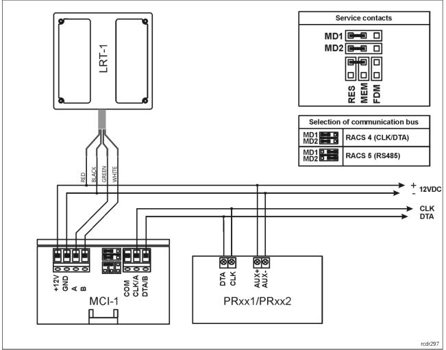
Fig. 8 Connection of LRT-1 reader to PRxx1 or PRxx2 access controller
