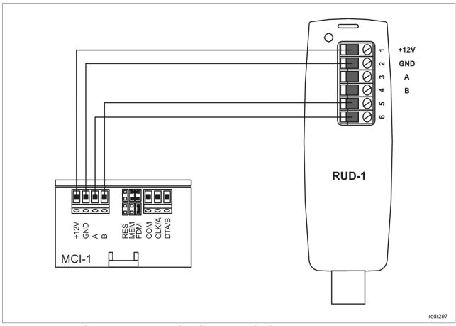
Fig. 6 Connection of MCI-1 to RUD-1 interface (firmware update)
