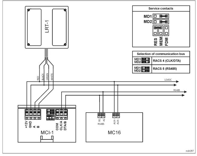
Fig. 7 Connection of LRT-1 reader to MC16 access controller
