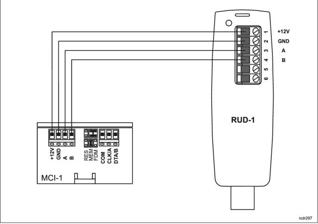
Fig. 5 Connection of MCI-1 to RUD-1 interface (configuration)
