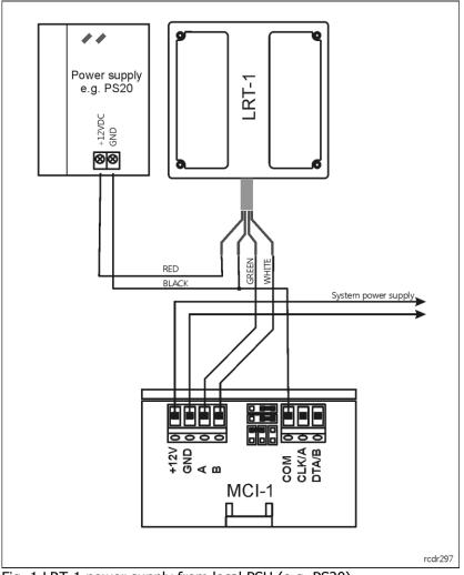
Fig. 1 LRT-1 power supply from local PSU (e.g. PS20)
