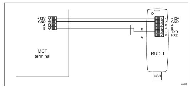
Fig. 7 Connection to RUD-1 interface (firmware update)
