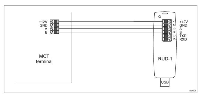
Fig. 6 Connection to RUD-1 interface (low level configuration)
