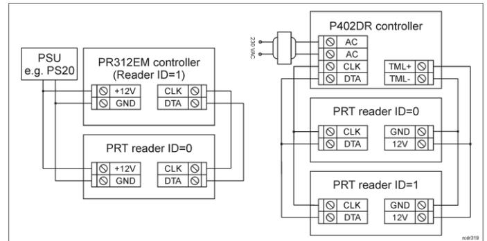
Fig. 1 Connection of PRT readers in RACS 4 system (examples)
