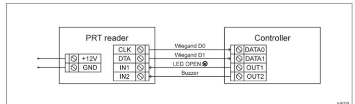
Fig. 2 Connection of reader to controller via Wiegand interface
