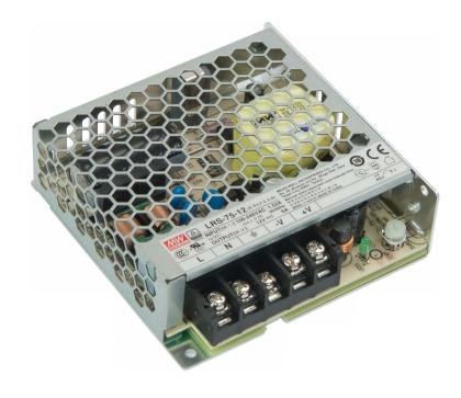
PS4D is LRS-75-12 (Mean Well) power supply unit with rated output voltage increased from 12.0 V to 13.8 V by means of original output potentiometer. PS4D is dedicated to installation in RACS 5 system, particularly to supply MCX2D and MCX4D expanders and PSD4D power distributors but it can also be used for other applications if its nominal conditions of use are satisfied. The PSU is
