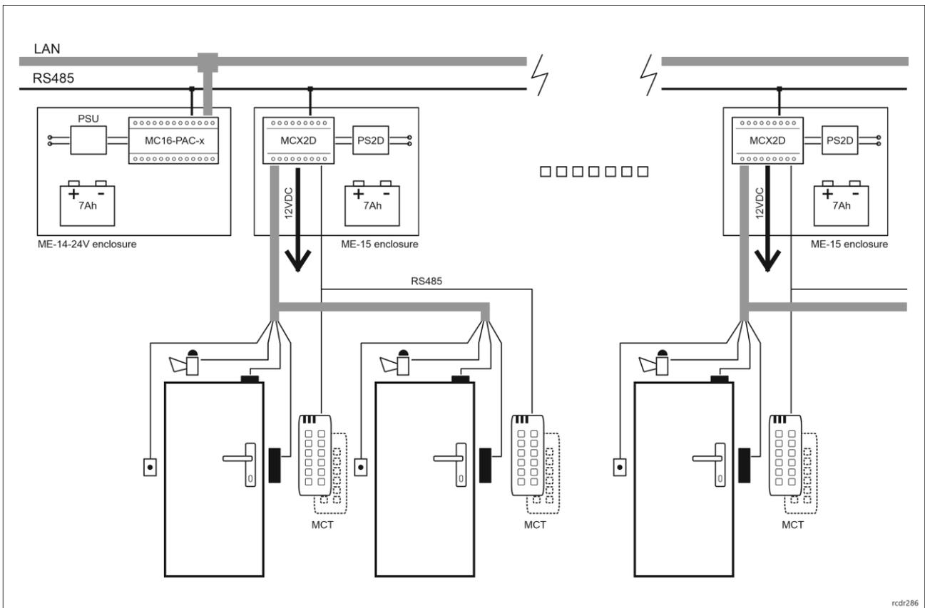
Fig. 5 Scenario of operation with multiple MCX2D expanders
