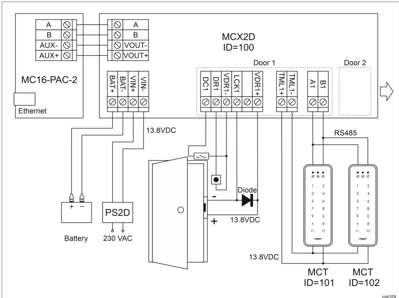
Fig. 6 Connection diagram for MCX2D expander in MC16-PAC-2-KIT
