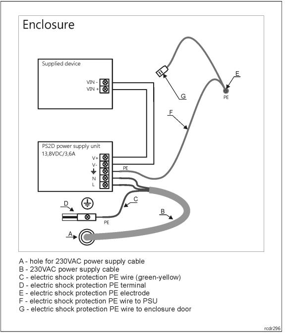
Fig. 1 PS2D installation inside enclosure
